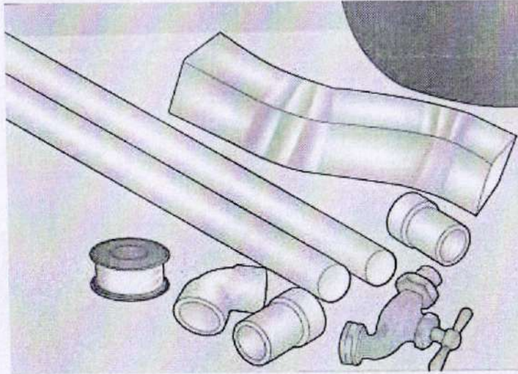
02) Pipes for Rainwater collection from terrace area
